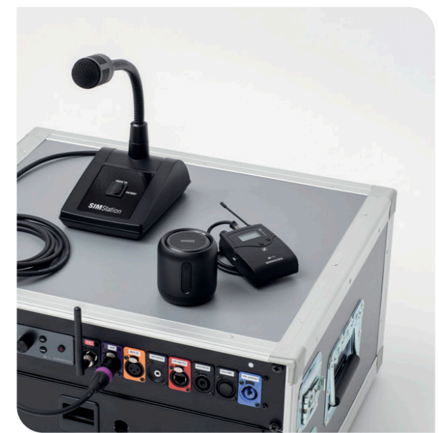
VOP - Voice of Patient: This allows you to simulate a patient voice in the training room. The connection can be made by radio or LAN
